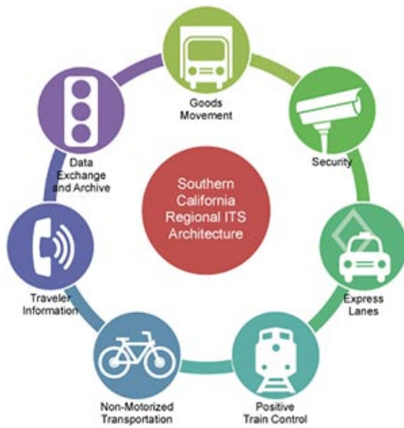
Figure 2: Architecture Elements ITS [14].
